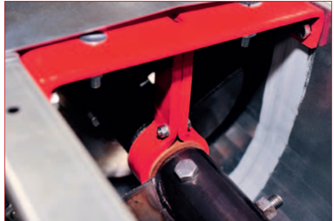
Fabricated hanger bearings use oil-impregnated wood inserts for easy installation and minimum maintenance.
